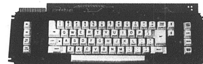
4. Two custom chips are all the electronics this Keytronics capacitive keyboard needs; 12 driver lines and eight receiver lines provide 98 possible matrix points for keys. The chips are built with integrated injection logic.
